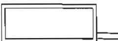
3. Make 45 degree bend on all edges. Make right angle bend on a strip.
